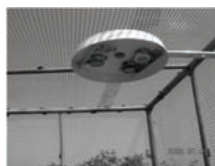
Monitoring of SO 2 , NO 2 & O 3 using Passive Samplers
