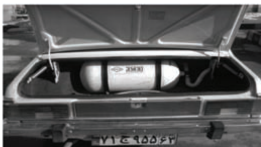
DUAL-FUEL SYSTEM IN PAYKAN VEHICLE AND REPLACING GASOLIN WITH CNG IN VEHICLES
